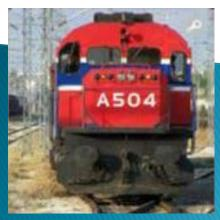
Power: 3.000hp  $(2.240kW) \sim 3.600hp$ (2,680 kW) **Drive Shafts** number: 6
