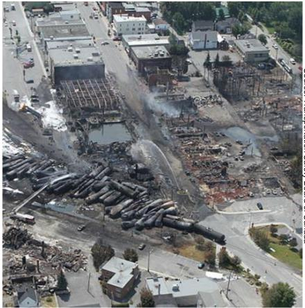
Occurred when maintenance crew failed to complete inspection and identify heat-related rail buckling, causing derailment.
